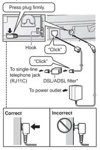
\*DSL/ADSL filter (not supplied) is required if you have DSL/ADSL service.
