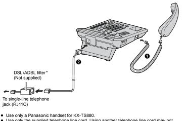
Use only the supplied telephone line cord. Using another telephone line cord may not allow the unit to work properly.
