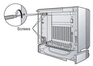
3. Pull the release lever in the direction of the arrow to disconnect the PSU from the back board.
