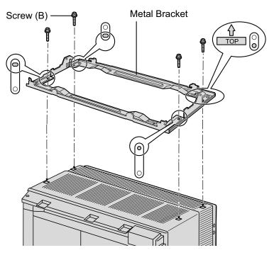
3. Lift Expansion Shelf 1, attach it to the metal bracket on the Basic Shelf, and slide it backwards until it locks.
