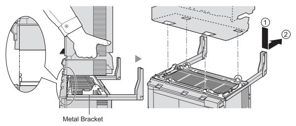
2. Secure Expansion Shelf to the metal bracket 2 with 2 screws (B).
