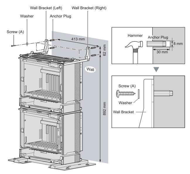
**4.** Check that the shelves are standing exactly vertically. If the shelves are leaning slightly to one side, move the base stands to adjust the position. (Since the base stands are attached loosely to the floor, it should be possible to adjust the position of the shelves.)
