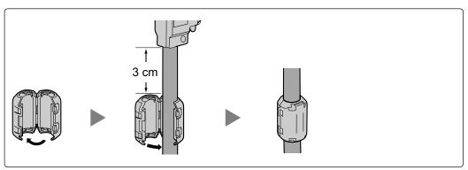
If you need to open the ferrite core, use a flathead screwdriver to unlatch the case of the ferrite core.
