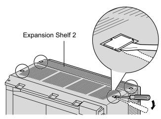
2. Fix the metal bracket to Expansion Shelf 2 with 4 screws (B).
