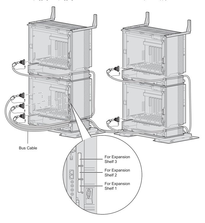
**6.** Attach the noise shield wires of each Bus Cable to the Basic Shelf and each Expansion Shelf with the screws of the BUS-M card.
