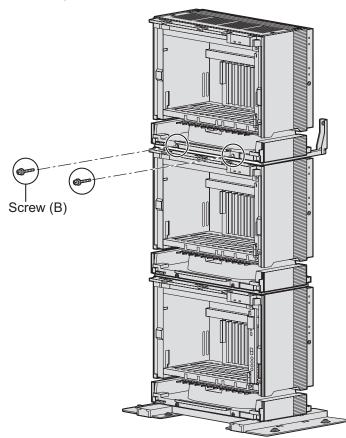
Installation of a 3-shelf system is complete. Next, it is necessary to connect the shelves. If you are installing a 4-shelf system, follow the procedure below before connecting the shelves.
