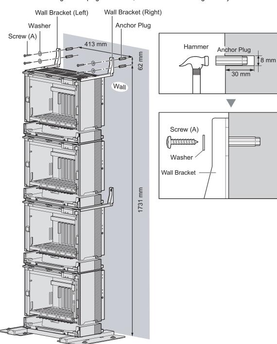
2. Check that the shelves are standing exactly vertically. If the upper shelves are leaning slightly to one side, move Expansion Shelf 3 to adjust the position. (Since the wall brackets are attached loosely to Expansion Shelf 3, it should be possible to adjust the position of the shelves.)
