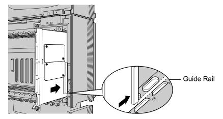
**3.** Push the release lever in the direction of the arrow so that the BUS-M card engages securely with the connector on the back board.
