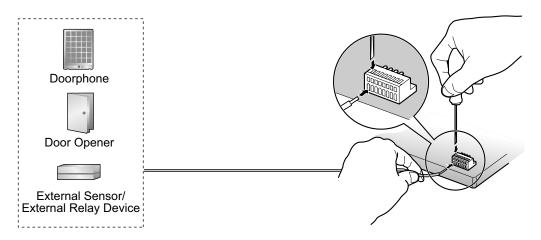
2. Attach the terminal blocks to the connectors of the DPH4/DPH2/EIO4 card on the PBX.
