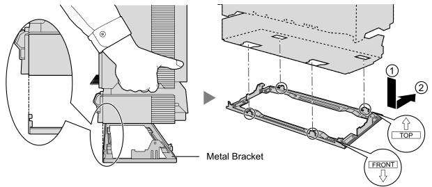
3. Secure the Basic Shelf to the metal bracket with 2 screws (B).
