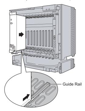
**2.** Push the release lever in the direction of the arrow, so that the PSU engages securely with the connector on the back board.
