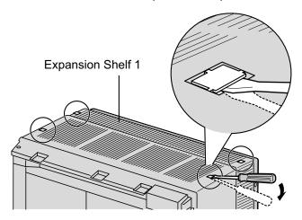
**3.** Fasten the wall brackets loosely to Expansion Shelf 1 with 4 screws (D). (This makes it easy to adjust the position of the shelves later.)
