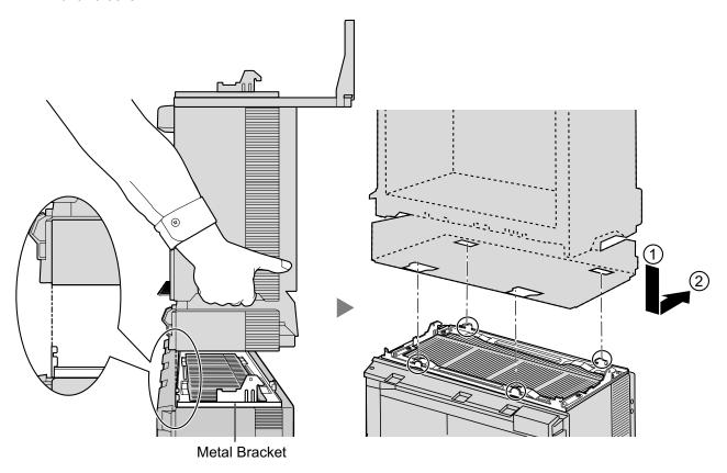
**6.** Secure Expansion Shelf 3 to the metal bracket with 2 screws (B).
