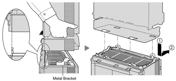
**4.** Secure Expansion Shelf 1 to the metal bracket with 2 screws (B).
