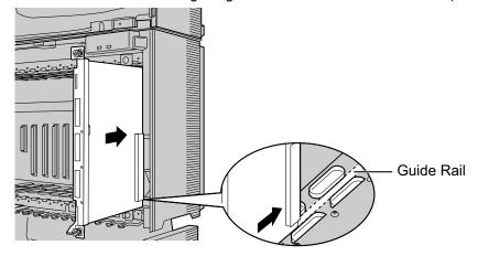
2. Push the release lever in the direction of the arrow so that the BUS-M card engages securely with the connector on the back board.
