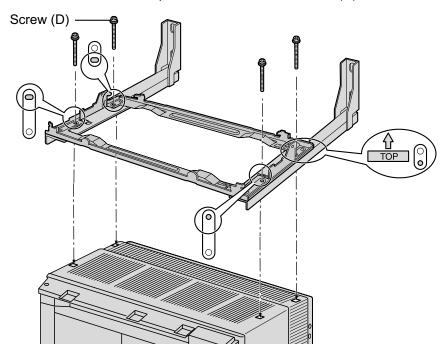
2. Fix the metal bracket to Expansion Shelf 1 with 4 screws (D).
