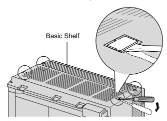
2. Fix the metal bracket to the Basic Shelf with 4 screws (B).
