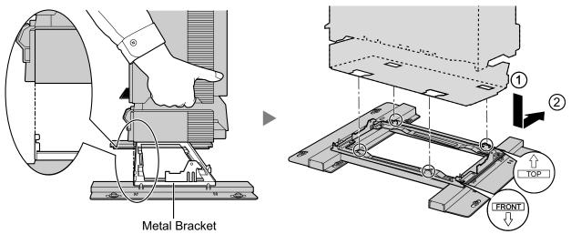
8. Secure the Basic Shelf to the metal bracket with 2 screws (B).
