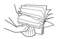
Pinch the right side of the recording paper guide (②), then slide it to match the paper size mark.
