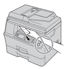
• Do not open the paper input tray before opening the left cover as the jammed paper may be pulled and the jam may get worse.
