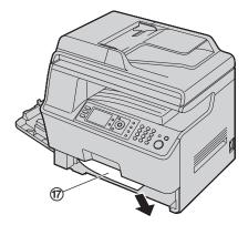
**3.** Insert the standard input tray into the unit, lifting the front part of the tray. Then push it completely into the unit.
