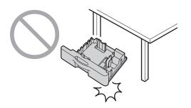
• Hold the lower input tray with both hands when removing or installing. The lower input tray weighs approximately 4.8 kg when fully loaded with recording paper.
