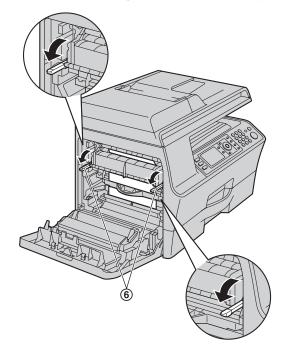
2. When the recording paper has jammed inside the fuser unit:
