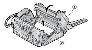
**5** Clean the thermal head (①) with a cloth moistened with isopropyl rubbing alcohol, and let it dry thoroughly.
