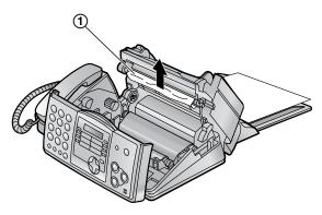
**5** Turn the gear with the blue core (①) in the direction of the arrow.
