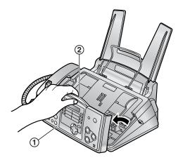
3 Clean the document feeder rollers (①) and rubber flap (②) with a cloth moistened with isopropyl rubbing alcohol, and let all parts dry thoroughly. Clean the glass (③) with a soft, dry cloth.
