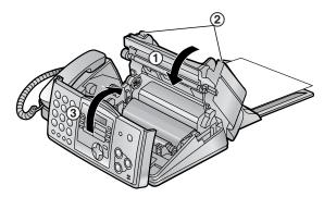
7 Remove the recording paper and straighten. Pull the tension plate forward (①) and hold open while inserting the paper.
