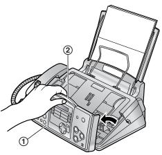
Release the back cover by pushing the green button (①) on the right side of the unit.
