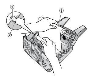
**5** Turn the gear with the blue core (①) in the direction of the arrow.
