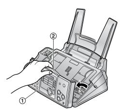
2 Release the back cover by pushing the green button (①) on the right side of the unit. OR
