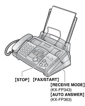
Set the fax machine to TEL mode by pressing [RECEIVE MODE] (KX-FP343)/[AUTO ANSWER] (KX-FP363) repeatedly to display the following.
