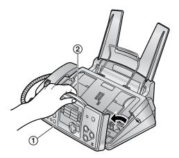
Release the back cover by pushing the green button (①) on the right side of the unit.OR
