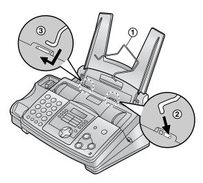
• The recording paper will be ejected from the top of the unit after printing. The recording paper support prevents the printed paper from curling.
